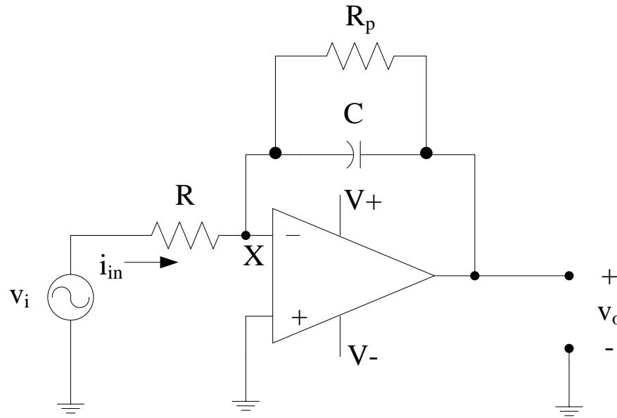
$$\begin{aligned}V_o &= -\left(\frac{Z_C // R_p}{R}\right)V_i \\&= -\left(\frac{V_i}{R}\right) \times \frac{R_p}{j\omega R_p C + 1}\end{aligned}$$
