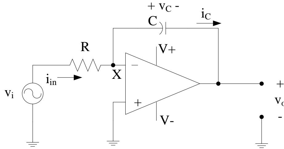
$$\begin{aligned} V_o &= -\left(\frac{Z_C}{R}\right)V_i \\ &= -\left(\frac{V_i}{R}\right) \times \frac{1}{j\omega C} \end{aligned}$$
